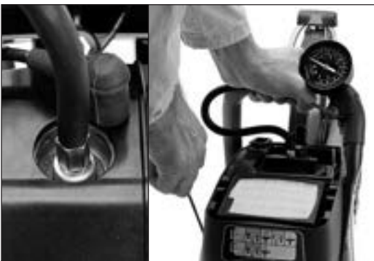
New, run-in engine approximately 10 bar Rectify below 8 bar
