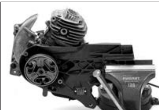
New, run-in engine approximately 10 bar Rectify below 8 bar
