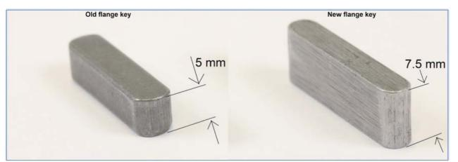
Figure 4 Flange keys. The old design to the left and the new to the right.
