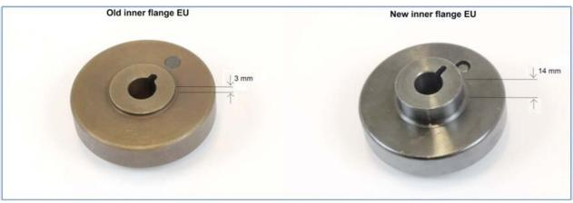
Figure 2: Inner flanges EU. The old design to the left and the new to the right.
