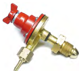
High volume compact regulator for propane. Ideal for appliances with a high throughput such as forced air heaters, bitumen boilers etc. 77kW with 4.8mm bore hose 87kW with 6.3 or 8mm hose when operated at 1 bar
