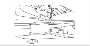
2. Fit the centre belt in position on the centre pulley.
