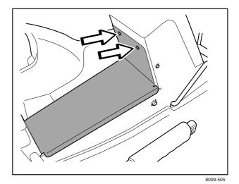
Check the tension of the steering cables by squeezing the cables together (at the arrows). It should be possible to squeeze the cables so that the distance between them is half the size, without using too much force.
