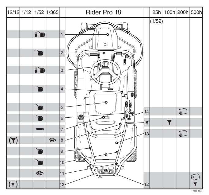
The position numbers for the lubrication points refer to the lubrication instructions on the following pages.
