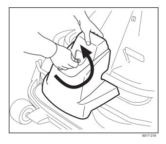
3. Loosen the two anti-scalp rollers, located under the front cover.
