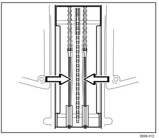
3. If necessary, the wires can be adjusted by tightening the adjuster nuts on each side of the steering collar.
