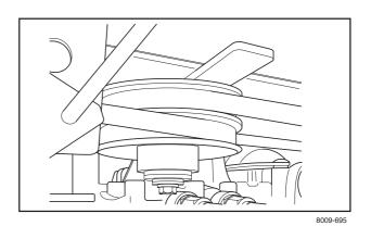
Reset the cutting unit in the mowing position. Make sure that the tongue (3) mates with the loop on the underside of the machine.
