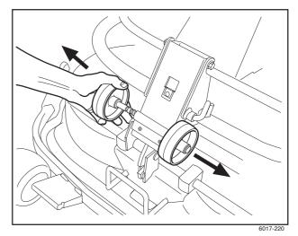
4. Fit the two anti-scalp rollers on each side of the cutting unit's rear section.
