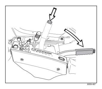
4. Select the required cutting height (1-7) using the cutting height lever.
