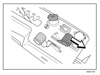
3. When the Rider is at a standstill, hold down the parking brake (1) and press in the lock button (2).
