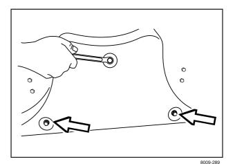
Removal of BioClip plug
