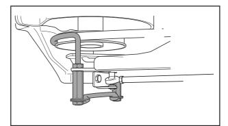
4. Check and adjust the belt tensioner. This is especially important when fitting a new belt, since stretching of the old belt may have been compensated for by changing the setting of the belt adjuster.
