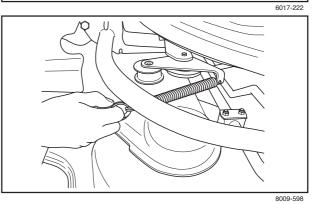
6. Put your foot on the front edge of the cutting unit next to the wheel and lift the cutting unit's front edge to make it easier to loosen the height adjustment stay.
