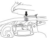
3 Press in the lock, grasp the pipes and slide in the cutting deck.
