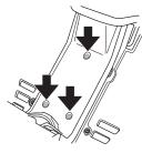
2 Check the tension of the steering wires by squeezing them together by the arrows as illustrated.
