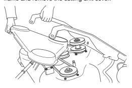
7 Loosen the spring that tensions the V-belt and pry off the helt
