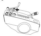
For cold starting the lever is moved backwards to its end position.
