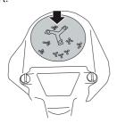
A blocked cooling intake will interfere with the cooling of the engine, which can damage the engine.
