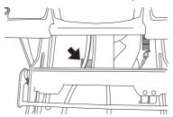
4 Push the deck in and put the front guide plugs in the grooves on the equipment frame, one on each side.
