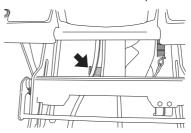
6 Grip the front edge of the unit and pull forwards until it stops.
