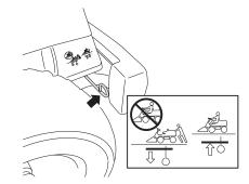
• Pull out the control to disengage the drive system.
