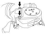
2 Loosen the hose clip that holds the filter cartridge.
