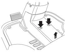
2 Check the tension of the steering wires by squeezing them together by the arrows as illustrated. It should be possible to push them together so that the distance between them is half as much, without using unnecessary force.
