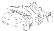
The Combi-unit, equipped with a BioClip-plug, finely chops the cuttings to fertiliser. Without the BioClip-plug the unit works in the same way as a rear ejection unit.
