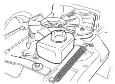
**Rider 220T** Fill if necessary with engine oil SAE 10W/40 (class SF–CC).
