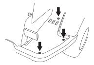
2 Loosen the locking nuts (1).
