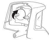
6 Fit the lamp holder in the lower slots on the servo housing.
