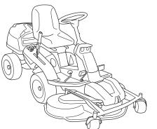
The machine 322T AWD are equipped with all wheel drive, chronometer and lights.
