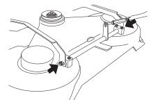
6 Remove the bolt so the track rod is released in one end.
