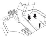
Check the tension of the steering wires by squeezing them together by the arrows as illustrated. It should be possible to push them together so that the distance between them is half as much, without using unnecessary force.
