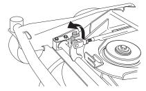
3 Remove the bolt so the track rod is released in one end.
