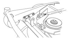
4 Unscrew the bolt holding the unit frame bracket.
