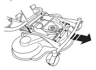
8 Lift the unit until it stops and a clicking sound is heard. The unit locks automatically in the vertical position.
