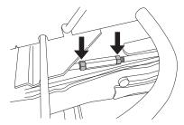
3 Screw out (extend) the stay to raise the rear edge of the cover.
