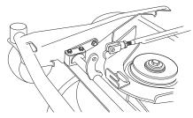
7 Remove the screws on the cutting cover. Lift the unit frame and remove the cutting unit cover.
