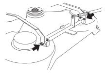
6 Remove the bolt so the track rod is released in one end.
