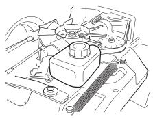
**Rider 316T** Fill if necessary with engine oil SAE 10W/40 (class SF–CC).
