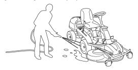
Oily dirt can be removed using a cold degreasing agent. Spray on a thin layer.
