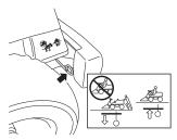
2 Lift up the cutting unit by pulling the lever backwards to locked position (transport position) and apply the parking brake. The engine can not be started if the parking brake is not pressed down.
