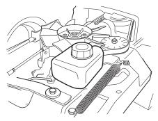
Fill if necessary with engine oil SAE 10W/40 (class SF–CC).
