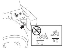
· Pull out the control to disengage the drive system.
