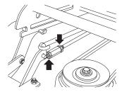
3 Screw out (extend) the stay to raise the rear edge of the cover.
