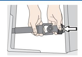
Remove the propeller shaft
