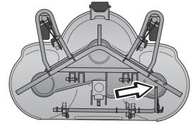
Adjustment screw tilt angle
