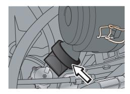
Particle trap on air filter
