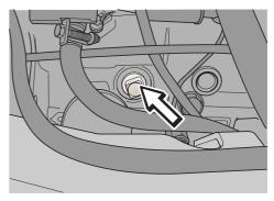
Coolant draining engine block
