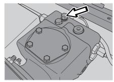
Unscrew the bypass valve when towing
