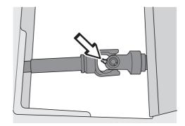
Propeller shaft's joints
