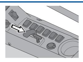
Engine speed control in idling mode
