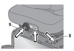
Lateral adjustment and adjusting suspension
