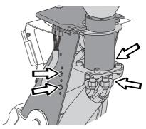
Adjusting the steering column vertically.
