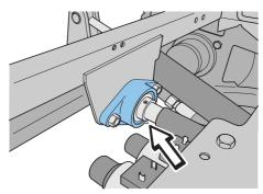
The power take-off shaft's front support bearing
