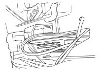
5 Remove the cooling fan, it is held in place by a nut.
