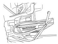
6 Remove the cooling fan, it is held in place by a nut.
