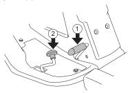
3 Press in the lock button on the mechanical lifting lever and lower the cutting unit.
