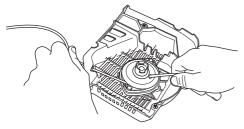
Secure the starter cord around the cord pulley as illustrated. Tighten the fastening well and ensure that the free end is as short as possible. Secure the end of the starter cord in the starter handle.
