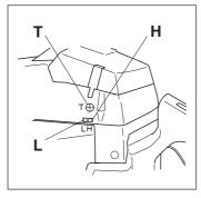
• The T screw regulates the idling speed. If the screw T is turned clockwise this gives a higher idling speed; counter-clockwise a lower idling speed.
