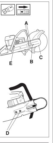
WARNING! Never use a power cutter without a blade guard over the cutting blade.
