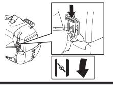
WARNING! When the engine is started with the choke in choke position the cutting attachment will start to rotate immediately.
