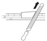
File all the teeth to the same length. When the length of the cutting teeth is reduced to 4 mm (5/32") the chain is worn out and should be replaced.
