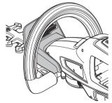
Check that the hand guard is fitted correctly. Check that the hand guard is undamaged.
