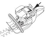
**CAUTION!** The stop switch automatically returns to the start position. In order to prevent unintentional starting, the spark plug cap must be removed from the spark plug when assembling, checking and/or performing maintenance.
