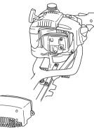
Some mufflers are equipped with a special spark arrestor mesh. If your machine has this type of muffler, you should clean the mesh at least once a week. This is best done with a wire brush.
