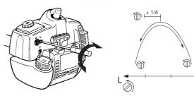
**CAUTION!** If the blades move while the engine is idling the T screw should be turned anti-clockwise until they stop.
