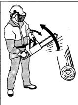
If the kickback is less violent or the kickback zone of the bar is closer to you the chain brake will be activated manually by the movement of your left
