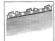
2 Keep the chain cutting teeth properly sharpened! Follow our instructions and use the recommended file gauge. A damaged or badly sharpened chain increases the risk of accidents.
