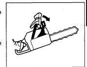
3 You can also use the chain brake as a temporary brake when you change position or if you put the saw down for a short time. You should also apply the chain brake manually if there is a risk of the chain accidentally hitting anyone or anything close by.
