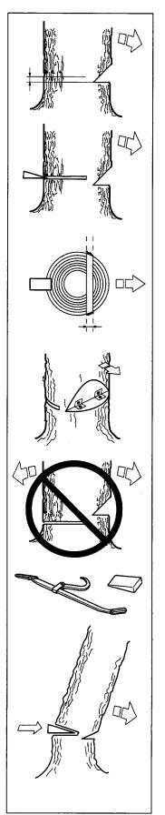
We recommend that you use a bar that is longer than the diameter of the tree, so that you can make the FELLING CUT and DIRECTIONAL CUT with single cutting stokes. (See "Technical data" to find out which lengths of bar are recommended for your saw).
