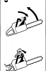
During felling your left hand grasps the front handle in such a way that it cannot activate the safety trigger. In this position the chain brake can only be activated by the inertia action of the counterweight.
