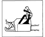
5 As mentioned in section A, kickback can be very sudden and violent. Most kickbacks are minor and do not always activate the chain brake. If this happens you should hold the chain saw firmly and not let go.
