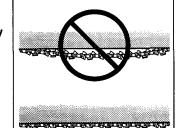
Keep cutting equipment well lubricated and properly maintained! A poorly lubricated chain is more likely to break and lead to increased wear on the bar, chain and drive sprocket.
