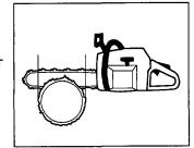
There are methods for felling trees with a diameter larger than the bar length. However these methods involve a much greater risk that the kickback zone of the bar will come into contact with the tree.
