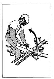
4 Never use the saw above shoulder height and try not to cut with the tip of the bar.
