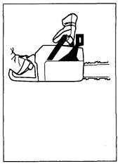
The way the chain brake is triggered, either manually or automatically, depends on the force of the kickback and the position of the chain saw in relation to the object that the kickback zone of the bar strikes.
