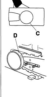
2 The safety trigger is designed solely to activate the chain brake. Another important safety feature is that it prevents the chain from hitting your left hand if you lose your grip on the front handle.
