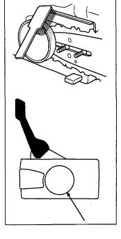
Regularly check that the brake band is at least 0.6 mm thick at its thinnest point.
