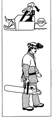
4 To release the chain brake pull the safety trigger backwards, towards the front handle.
