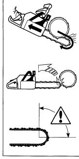
In this case the saw pulls itself towards the tree and the front edge of the saw provides a natural rest when cutting. Cutting on the pull stroke gives you better control over the saw and the position of the kickback zone.
