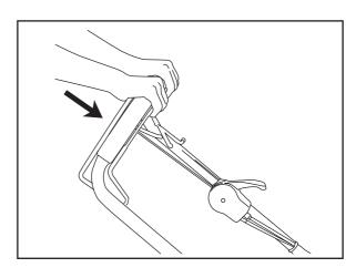
When finished mowing release OPC bail to stop blade rotation.
