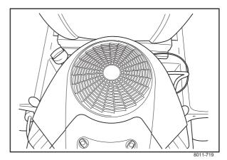
Check and clean the cooling air intake
