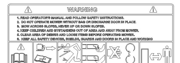
Read Operator's Manual. Shut off engine & remove spark plug wire before performing any maintenance or repair work.
