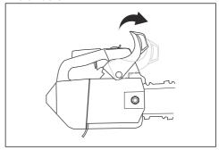
Push the air purge bulb about 6 times or until fuel starts to fill the bulb. It is not necessary to fill the air purge bulb completely.
