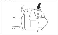
Make sure that the throttle trigger is locked at the idle position when the throttle trigger lockout is released.
