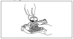
5. Remove the bolt in the center of the pulley and remove the pulley.
