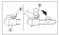
Pull the front hand guard rearward to disengage the chain brake.
