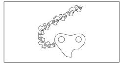
Bar groove width, in/mm. The groove width in guide bar must be the same as the chain drive links width.
