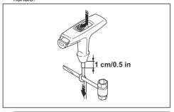
**Note:** If the starter rope is broken in the starter rope handle, push the starter handle cover down. Use the combination wrench to remove the starter handle cover
