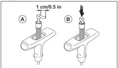
15. Pull the starter rope until 1 cm of the spring guide is shown. At the same time, assemble the starter handle cover.
