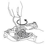
Undo the bolt in the centre of the pulley and remove the pulley.
