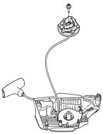
Hold the starter handle and pull the starter cord so that at least 10mm of the spring guide is visible. Press the starter handle cover at the same time and slide it out of the starter handle.
