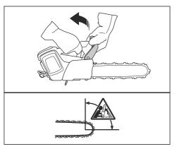
How the chain brake is engaged is in relation to the force of the kickback and the position of the product. If you get an intense kickback while the kickback zone is farthest away from you, the chain brake engages by the inertia release. If the kickback is small or the kickback zone is nearer you, the chain brake engages manually by your left hand.
