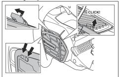
Push the air intake cover to the left until the holes align.
