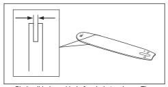
Chain oil hole and hole for chain tensioner. The guide bar must align with product.
