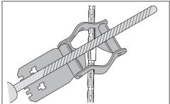
4. Remove material from one side of all the cutting teeth.
