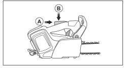
Make sure that the power trigger is locked at the idle position when the power trigger lockout is released.
