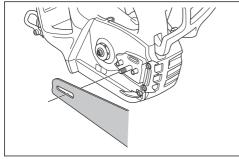
Steer the guide bar to its most rear position. Lift the saw chain above the drive sprocket and engage it in the groove on the guide bar. Start on the top edge of the guide bar.
