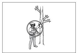
Do not try pruning or limbing operations if you do not have special training.  The vibration level increases if you cut with cutting equipment that is incorrect or not correctly sharpened. Cutting hardwoods, such as broadleaf trees, causes more vibration than cutting softwoods, such as conifers.
