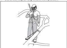
Do a check of the harness, belt and ropes at a regular interval.  If you must climb with the product, attach the product to the rear connection point on the harness. The rear connection point keeps the product clear from climbing lines and makes sure that the weight has central support down your spine.
