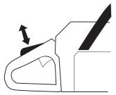
• Check that the throttle control and throttle lock move freely and that the return springs work properly.
