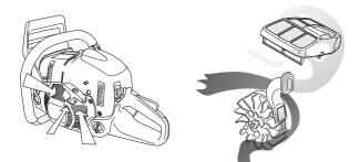
IMPORTANT! In order to maintain operation of the centrifugal cleaning system it must be regularly maintained. Clean the air intake to the starter, the fins on the flywheel, the space around the flywheel, inlet pipe and carburettor compartment.
