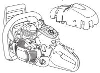
• Remove the air filter after taking off the air filter cover. When refitting make sure that the air filter seals tightly against the filter holder. Clean the filter by brushing or shaking it.
