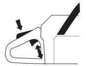
• Start the chain saw and apply full throttle. Release the throttle control and check that the chain stops and remains stationary. If the chain rotates when the throttle control is in the idle position you should check the carburettor idle adjustment.
