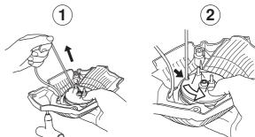
• Undo the screw in the centre of the pulley and remove the pulley. Insert and fasten a new starter cord to the pulley. Wind approx. 3 turns of the starter cord onto the pulley. Connect the pulley to the recoil spring so that the end of the spring engages in the pulley. Fit the screw in the centre of the pulley. Insert the starter cord through the hole in the starter housing and the starter handle. Make a secure knot in the end of the starter cord.
