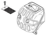
The muffler is designed to reduce the noise level and to direct the exhaust gases away from the operator. The exhaust gases are hot and can contain sparks, which may cause fire if directed against dry and combustible material.
