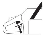
Press the throttle lock and make sure it returns to its original position when you release it.
