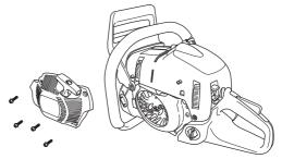
• Pull out the cord approx. 30 cm and hook it into the notch in the rim of the pulley. Release the recoil spring by letting the pulley rotate slowly backwards.
