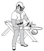
4 Never use the chain saw above shoulder height and try not to cut with the tip of the bar. Never use the chain saw one-handed!
