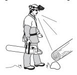
Take the utmost care when cutting through branches or logs that are in tension. A log or branch that is in tension can suddenly spring back into its natural position before or after you cut it. If you stand on the wrong side or start cutting in the wrong place it may strike you or your chain saw, so that you lose control. Both situations could cause serious injury.
