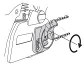
Fold the knob back in to lock the tensioning.
