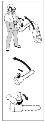
If the kickback is less violent or the kickback zone of the bar is closer to you the chain brake will be activated manually by the movement of your left
