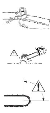
Two factors decide whether the chain will jam or the log will split. The first is how the log is supported and the second is whether it is in tension.
