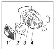
Clean the cooling system with a brush once a week, more often in demanding conditions. A dirty or blocked cooling system results in the saw overheating which causes damage to piston and cylinder.
