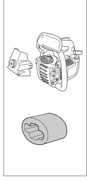
An air filter, which is used for some time, cannot be cleaned completely. Therefore it must be replaced by a new one, with regular intervals.
