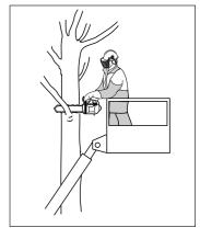
Take great care when you cut with the top edge of the bar, i.e. when cutting from the underside of the object. This is known as cutting on the push stroke. The chain tries to push the saw back towards the user.
