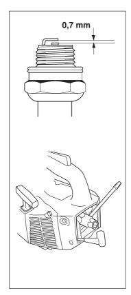
IMPORTANT! Always use the recommended spark plug type. An incorrect spark plug can severely damage the piston/cylinder.
