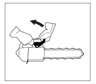
5 As mentioned in section A, kickback can be very sudden and violent. Most kickbacks are minor and do not always activate the chain brake. If this happens you should hold the chain saw firmly and not let go.
