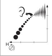
The H jet is correctly adjusted when the saw "4-strokes" slightly. If the saw "screams", it is set too lean. If smoke comes from the muffler while the saw is "4-stroking", it is set too rich. Turn the H needle clockwise to achieve a setting which sounds right.
