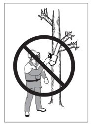
If it is necessary to cut branches or similar which are above shoulder height, a lift platform or scaffold tower is recommended.
