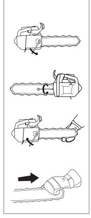
The position of the chain tensioning screw varies from model to model. See the" What is what" section to find out where it is on your saw.
