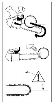
Cutting with the bottom edge of the bar, i.e. from the top of the object downwards, is known as cutting on the pull stroke. In this case the saw pulls itself towards the tree and the front edge of the saw provides a natural rest when cutting. Cutting on the pull stroke gives you better control over the saw and the position of the kickback zone.
