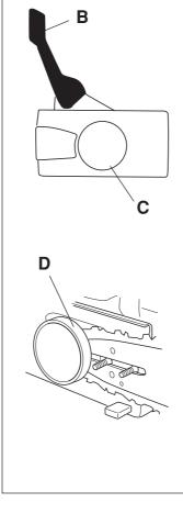
2 The front hand guard is not designed solely to activate the chain brake. Another important safety feature is that it prevents the chain from hitting your left hand if you lose your grip on the front handle.
