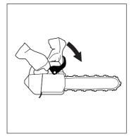
One-handed working may be necessary, but should only be carried by persons who are trained and have knowledge of tree maintenance work using a chain saw, both above and on the ground. **Do not let go of the handles!**
