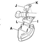
Remove the mounting plate (H). Fit the adapter (I) and bracket (J) with the two screws (K) as shown. Fit the blade guard (A) to the adapter using the 4 screws (L) as shown.
