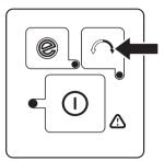
When the rotation button is pressed, the green diode will lit and the trimmer head rotates in counterclockwise. The trimmer head always rotates clockwise by default (green LED is off).
