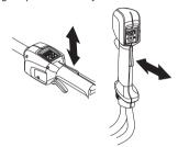
Check that the power trigger and the power trigger lockout move freely and that the return spring works properly.
