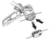
· Pull out the line chute assembly.
