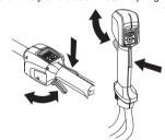
See instructions under the heading Start. Start the machine and apply full power. Release the power trigger and check that the cutting attachment stops and remain at a standstill.
