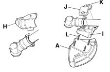
Remove the mounting plate (H). Fit the adapter (I) and bracket (J) with the two screws (K) as shown. Fit the blade guard (A) to the adapter using the 4 screws (L) as shown.
