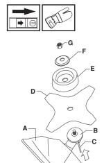
Hook the blade guard/combination guard (A) onto the fitting on the shaft and secure with the bolt.
