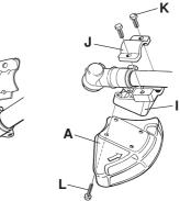
Remove the mounting plate (H). Fit the adapter (I) and bracket (J) with the two screws (K) as shown. Fit the blade guard (A) to the adapter using the 4 screws (L) as shown.
