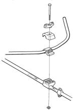
Put on the harness and hang the machine from the support hook. Now make a final adjustment so that the machine is in a comfortable working position when it hangs from the harness. Tighten the knob.
