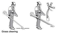
The machine should be supported in a harness when grass clearing so that the cutting equipment is parallel to the ground.
