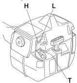
The L and H-jets are used to adjust the supply of fuel to match the rate that air is admitted, which is controlled with the throttle. If they are screwed clockwise the air/fuel ratio becomes leaner (less fuel) and if they are turned anti-clockwise the ratio becomes richer (more fuel). A lean mixture gives a higher engine speed and a rich mixture gives a lower engine speed.
