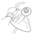
Fit the bottom half of the trimmer head (K) to the cover (I) by pressing them together, with the cut-outs on the bottom half aligned with the catches on the cover.
