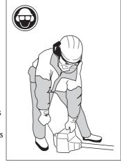
• Place the machine on the ground, ensure the cutting equipment runs free of twigs and stones. Push the machine body towards the ground using your left hand. (NOTE! Not with your foot). Grip the starter handle with your right hand and pull the starter cord.
