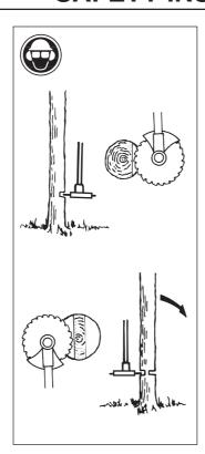
If the blade should jam in the stem, never jerk the machine free. If you do this the blade, angle gear, shaft or the handlebars can be damaged. Release the handlebars and grip the shaft with both hands and slowly pull the machine free.
