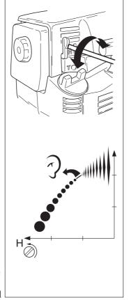
needle is adjusted correctly when the machine 'splatters' a little . If the machine smokes heavily at the same time as it 'splatters' heavily the adjustment is too rich.
