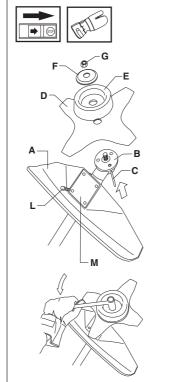
kpm). Use the socket spanner in the tool kit. Hold the handle of the spanner as close to the blade guard as possible. The nut is tightened when the spanner is turned against the direction of rotation (left-hand thread).
