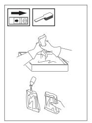
fitting the filter on the machine. Never use common engine oil. This would drain through the filter quite quickly and collect in the bottom.
