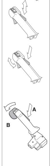
• See section "Start". Start the machine and apply full throttle. Release the throttle and check that the cutting equipment stops and remains at a standstill. If the cutting equipment rotates with the throttle in the idling position then the carburettor's idling setting must be checked. See chapter "Maintenance".
