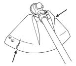
Check that the trimmer head and trimmer guard are not damaged or cracked. Replace the trimmer head or trimmer guard if they have been exposed to impact or are cracked.
