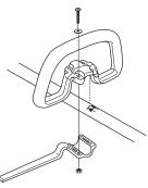
• Finely adjust the J-handle to give a comfortable working stance. Tighten the screws.
