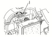
7 Bind the throttle cable (J) and the flexible shaft (K) with two bands (L).
