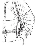
Check that the harness straps are correctly positioned. Once the harness and machine have been adjusted, check that the harness quick release works correctly.
