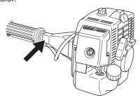
Using incorrectly wound cord or a blunt or incorrect cutting attachment (wrong type or incorrectly filed, see instructions under the heading Filing the blade) increases the level of vibration.
