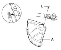
**142R:** Fit the guard (A) to the gear housing using the support plate (M) and two screws (L).
