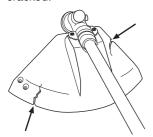
Check that the trimmer head and trimmer guard are not damaged or cracked. Replace the trimmer head or trimmer guard if they have been exposed to impact or are cracked.
