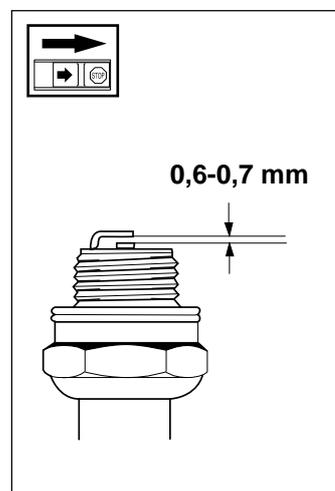
**If the machine is low on power, difficult to start or runs poorly while idling always check the spark plug first.**
