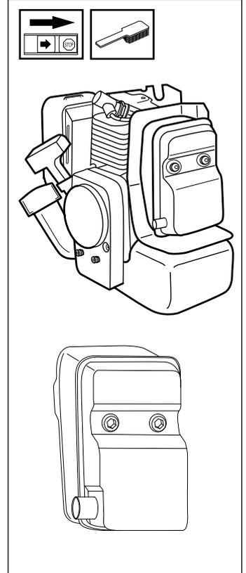
If the screen is frequently blocked, this can be a sign that the function of the catalytic converter is impaired. Contact your dealer to inspect the muffler. A blocked screen will cause the engine to overheat resulting in damage to the cylinder and piston. Also see under "Maintenance".
