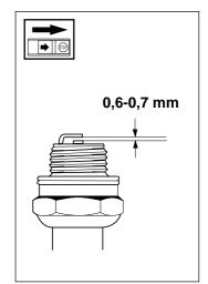
If the machine is low on power, difficult to start or runs poorly while idling always check the spark plug first.
