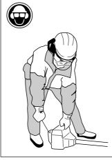
• Place the machine on the ground, ensure the cutting equipment runs free of twigs and stones. Push the machine body towards the ground using your left hand. (NOTE! Not with your foot). Grip the starter handle with your right hand and pull the starter cord.
