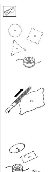
2)Keep the blade's teeth well and correctly sharpened! Follow our instructions and use the recommended filing gauge. An incorrectly sharpened or damaged blade increases the risk of an accident.
