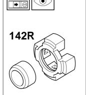
• Check that the vibration damping element is undamaged and securely attached.
