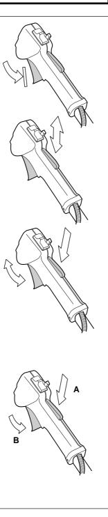
• See section "*Start*". Start the machine and apply full throttle. Release the throttle and check that the cutting equipment stops and remains at a standstill. If the cutting equipment rotates with the throttle in the idling position then the carburettor's idling setting must be checked. See chapter *"Maintenance"*.
