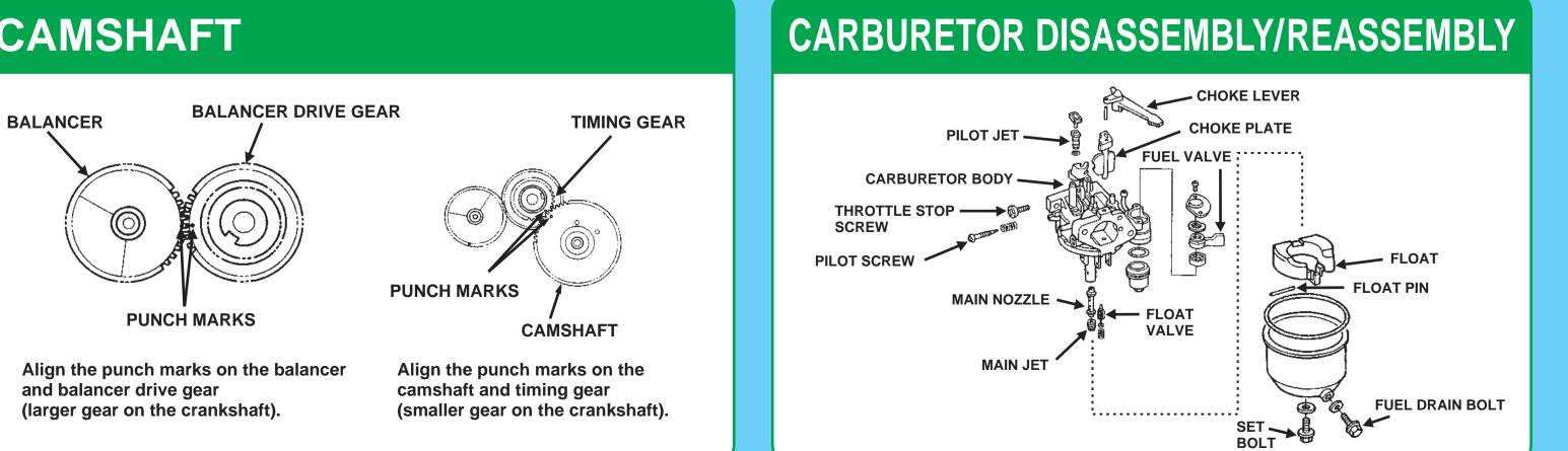
Align the punch marks on the balancer and balancer drive gear (larger gear on the crankshaft).
