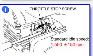
The standard idle speed may be different depending on the application. Refer to the equipment manufacturer's instructions for specific idle speed setting.
