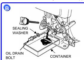
Drain the used engine oil while the engine is warm. Warm oil drains guickly and completely.
