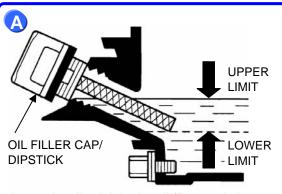
Insert the dipstick in the oil filter neck, but do not screw it in. Remove the dipstick and check the oil level.
