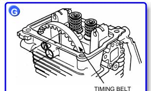
Check that the belt is not worn or cracked, and do not bend or twist the belt.
