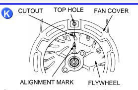
Set the piston at top dead center of the compression stroke (both valves fully closed).
