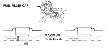
Refuel carefully to avoid spilling fuel. Do not fill the fuel tank completely. It may be necessary to lower the fuel level depending on operating conditions. After refueling, screw the fuel filler cap back on until it clicks.
