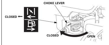
To restart a warm engine, leave the choke lever in the OPEN position.
