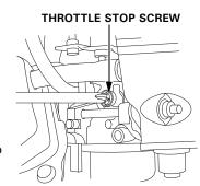
Standard idle speed: 1,400 +200 rpm
