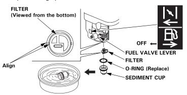
3. Reinstall the filter, new O-ring, and the sediment cup. Tighten the sediment cup securely.
