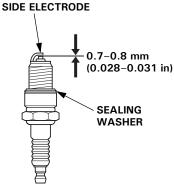
6. After the spark plug is seated, tighten with a 13/16-inch spark plug wrench to compress the sealing washer.
