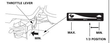
Some engine applications use a remote-mounted throttle control rather than the engine-mounted throttle lever shown here. Refer to the instructions provided by the equipment manufacturer.
