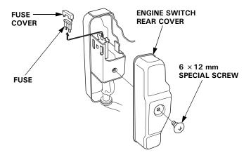
Frequent fuse failure usually indicates a short circuit or an overload in the electrical system. If the fuse burns out frequently, take the engine to a Honda servicing dealer for repair.
