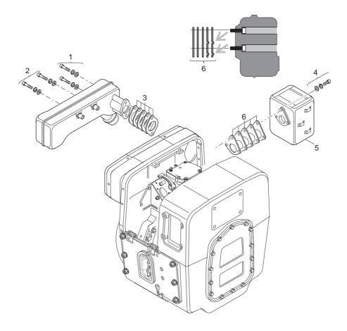
Sequence of dismantling the exhaust system:
