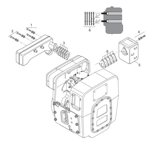
Sequence of dismantling the exhaust system:
